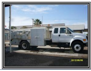
When this truck is transformed by our Firefighters into a Fire & Rescue Vehicle, it will carry up to 800 Gallons of water, firefighting foam, and our Technical Rescue Equipment, to include the large Spreaders, Cutters, Extending Rams, Air Bags and similar rescue gear already in our inventory.
